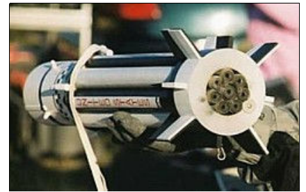
RIGHT: Tail end of Saturn motor cluster after 4th test flight. There appears to be some motor residue from blast deflection of the motor exhaust, but no damage from the Spider.
