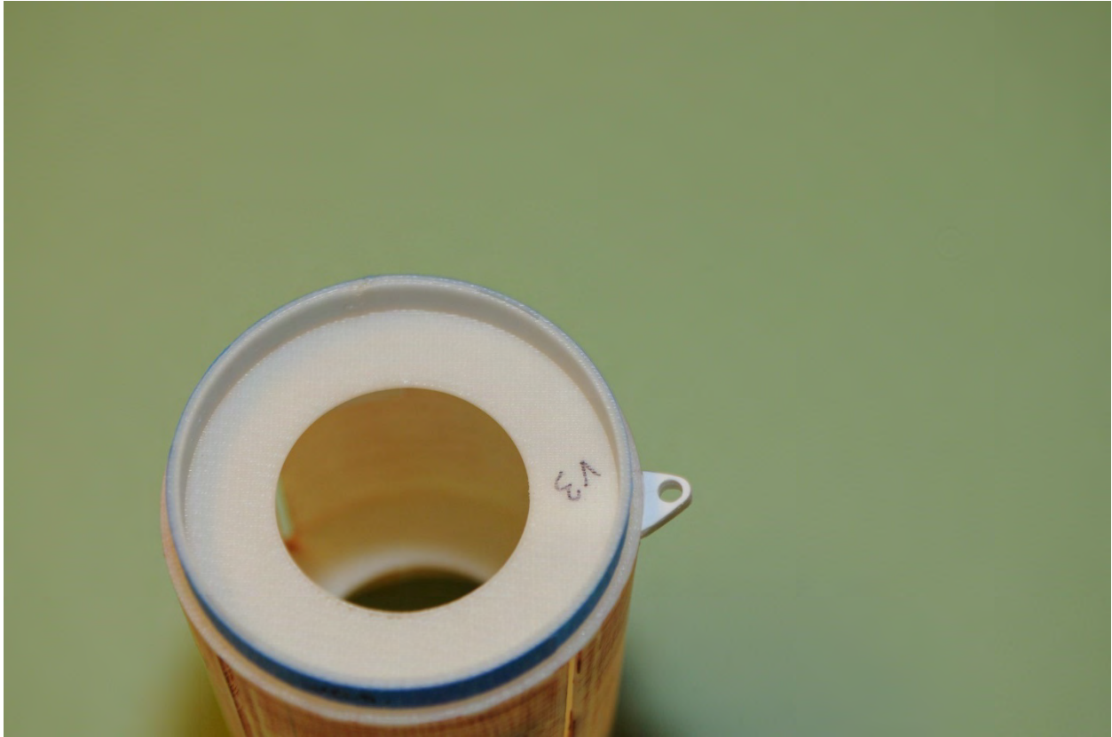
Photo 7: Tail Lug Installed
