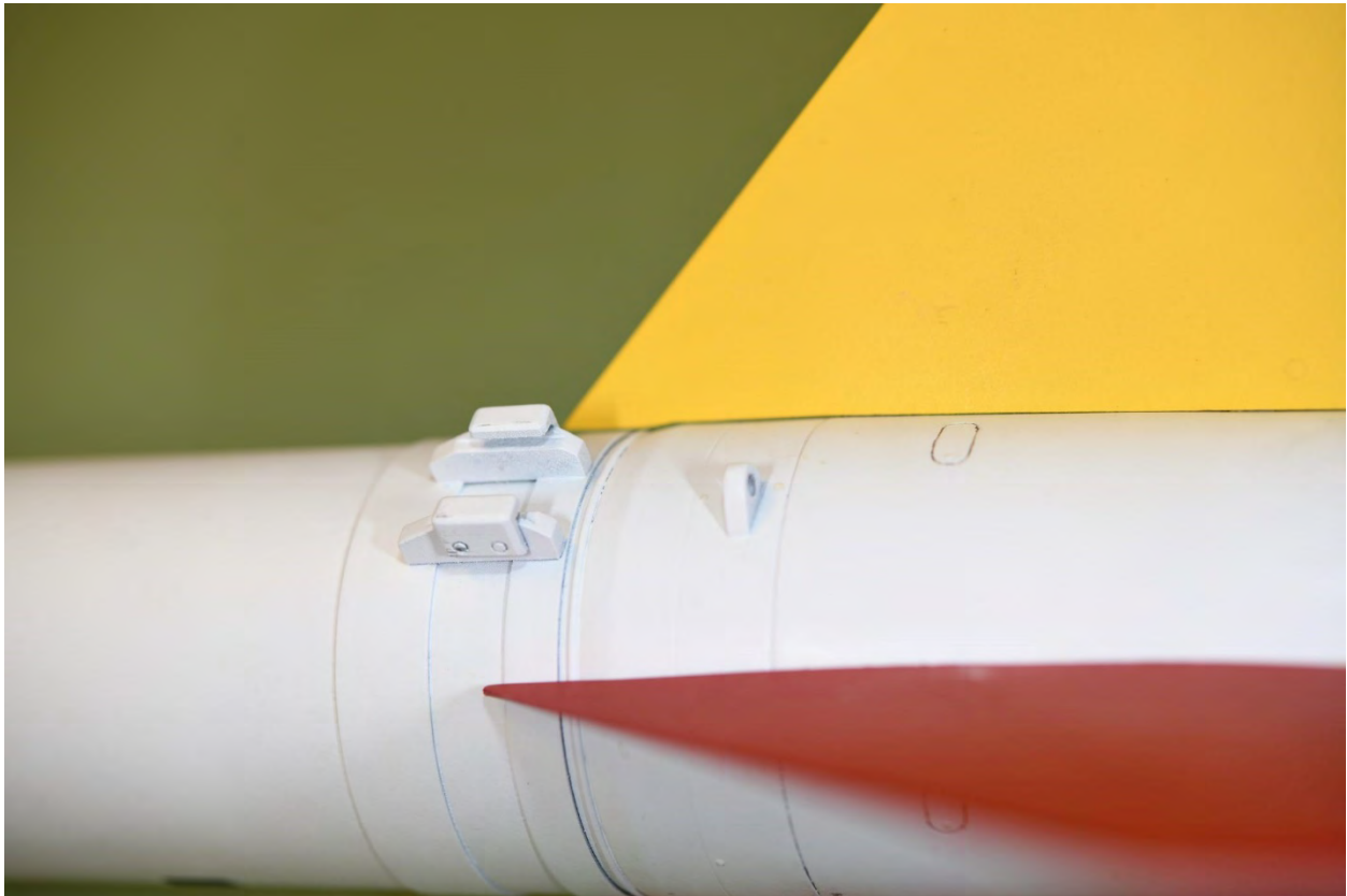
Photo 11: Aft Rail Lugs
