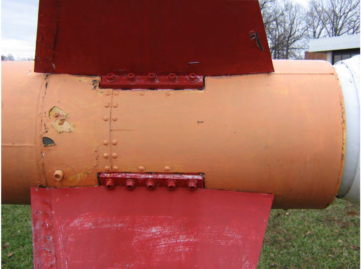
Photo 1: Nike Aft Nozzle Shrouds and Fin Bolting Arrangement
