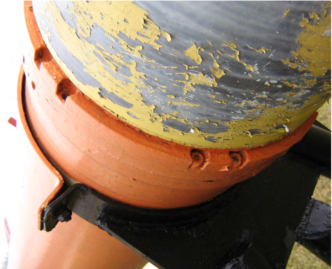
Photo 3: Nike Adapter Mounting Bolts
