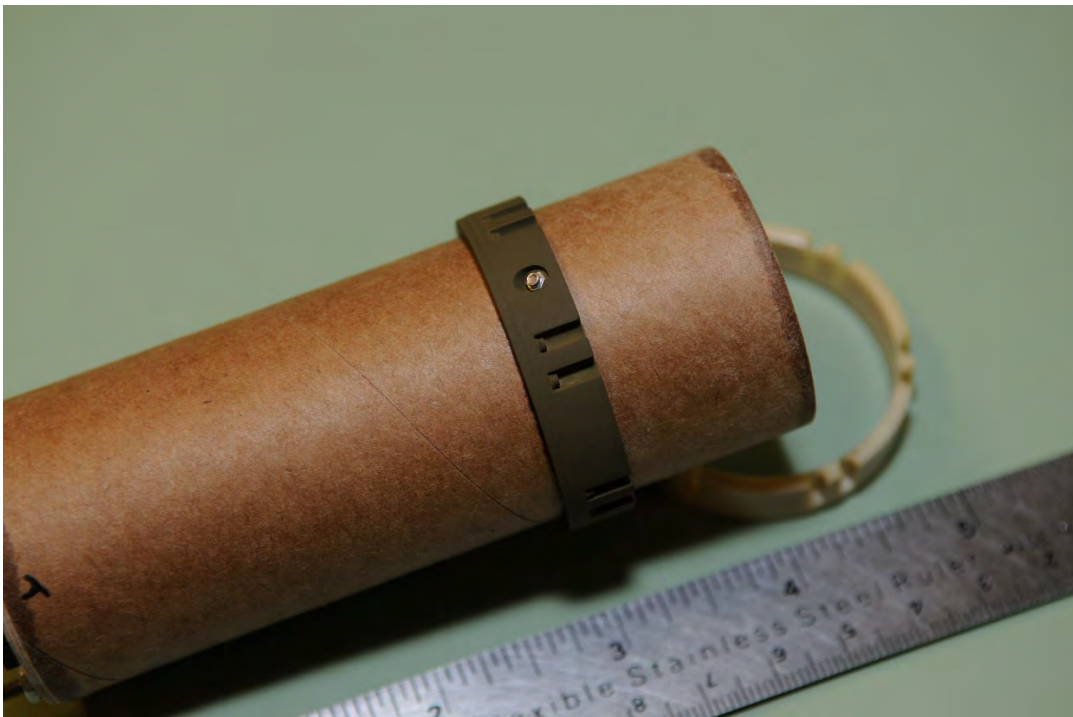
Photo 24: Umbilical Connector Installed
