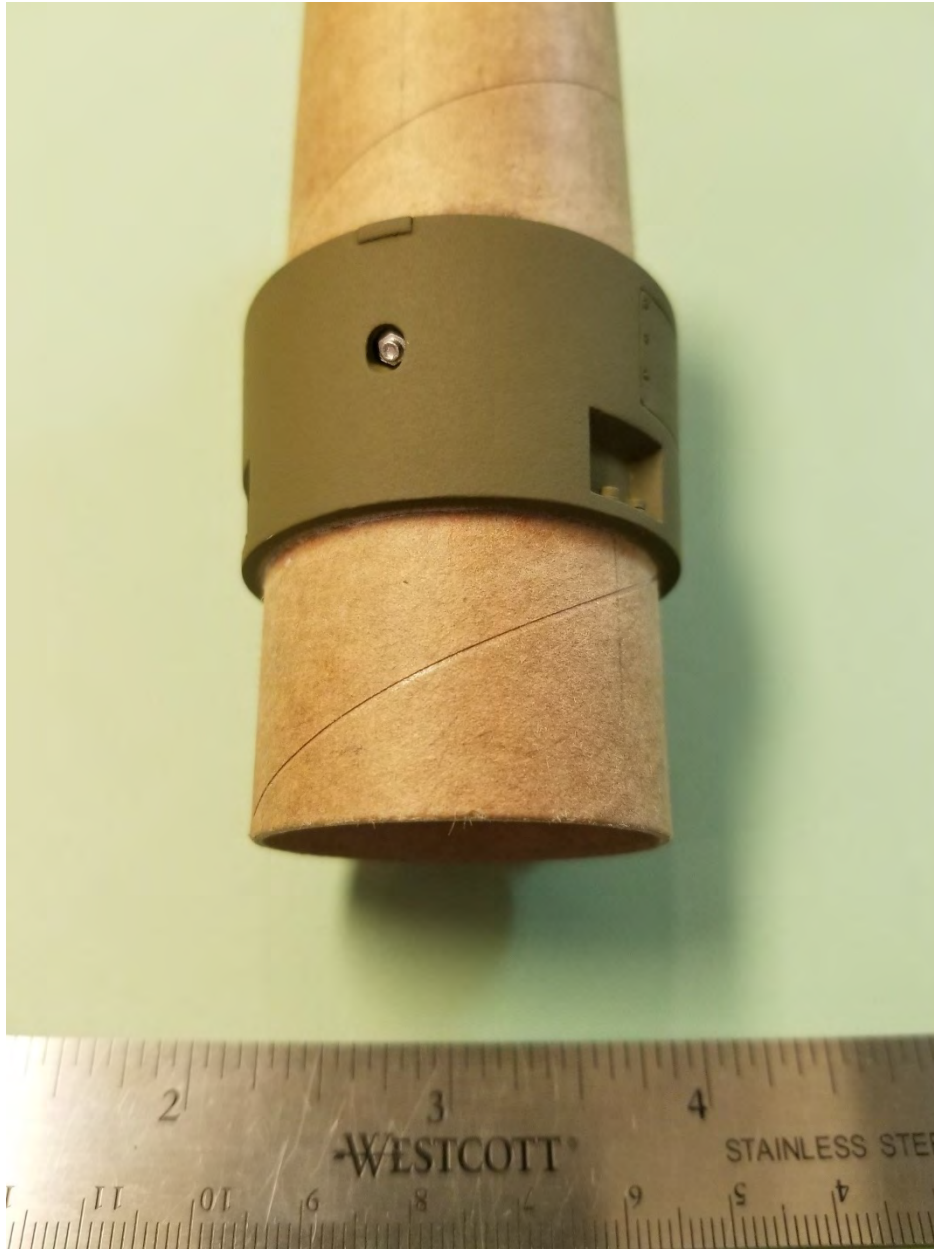
Photo 19: Umbilical Connector Installed
